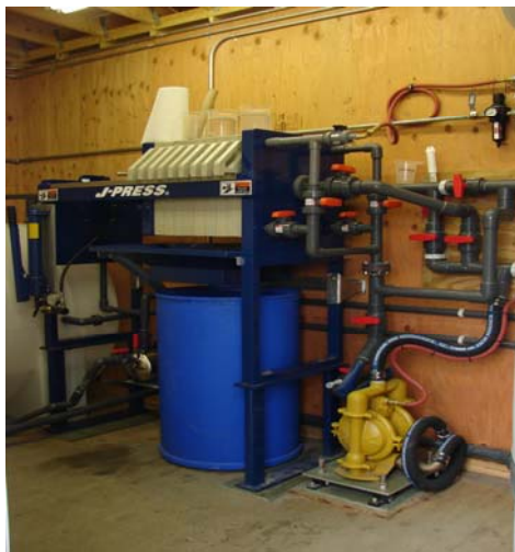
Figure 4 – Filter & Transfer Pump
